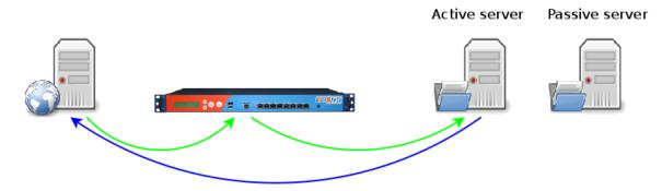
The client (here, the web server) pass through the **ALOHA** to access the NFS service. The NFS server talk directly to the client, bypassing the ALOHA load-balancer.
